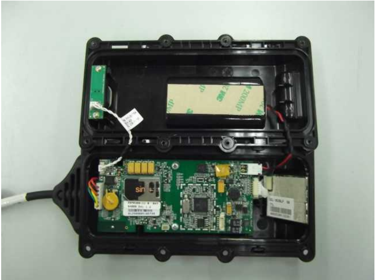
Picture 4. Internal View – GP battery
