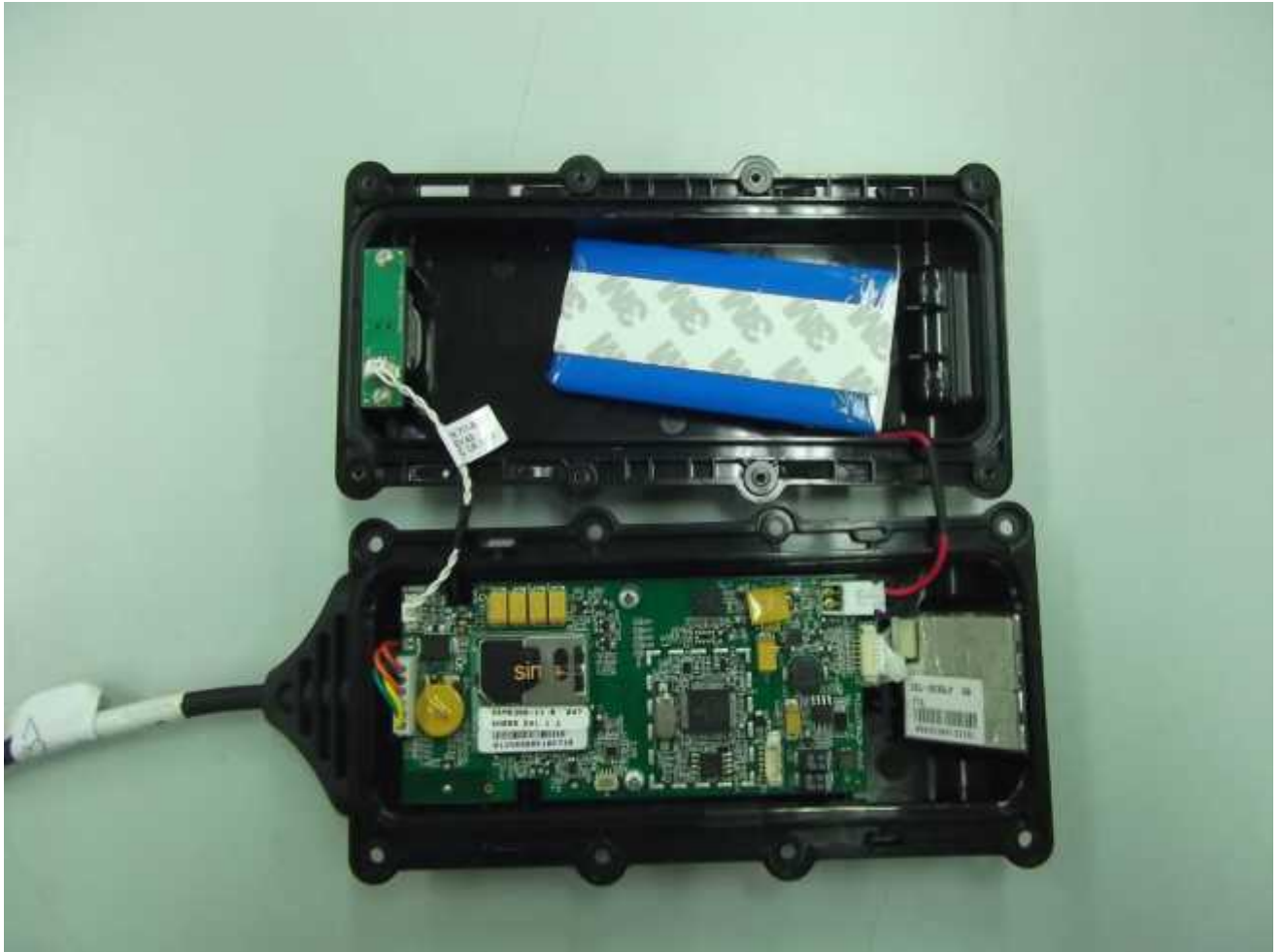
Picture 5. Internal View – Yoku battery
